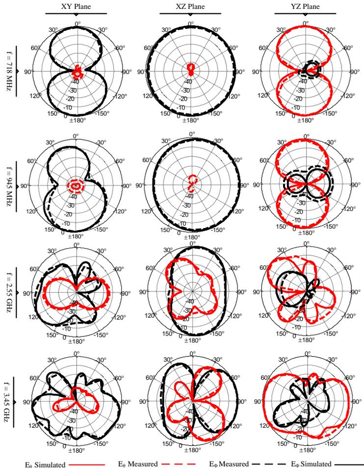
Fig. 7. Simulated and measured normalized radiation patterns
