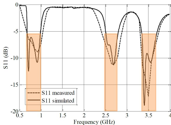
Fig. 5. Simulated and measured reflection coefficient
