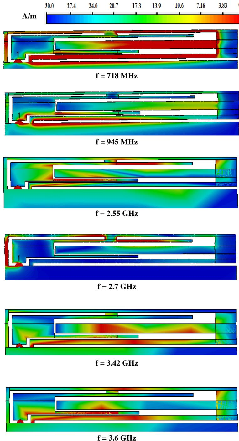
Fig. 3. Simulated surface current distribution
