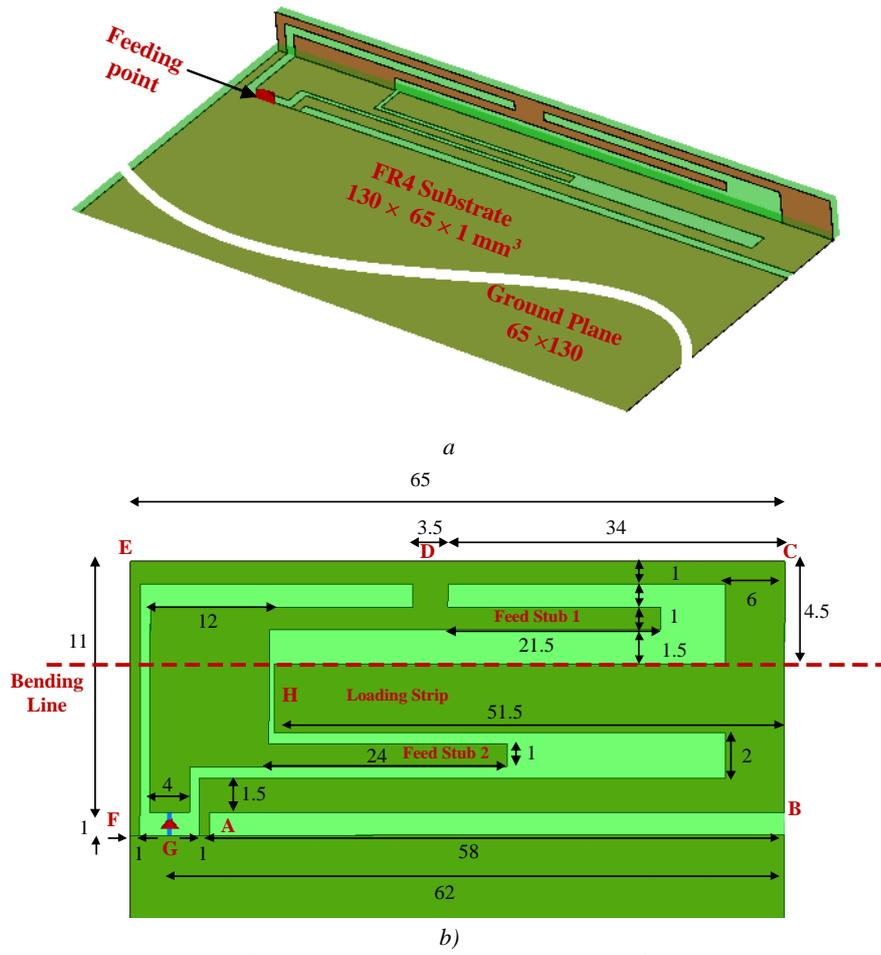
Fig. 1. a) Geometry of the proposed antenna, b) Dimensions of the proposed antenna
